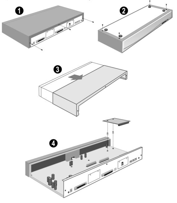
Caution: While installing, ensure that you wear a ground wrist strap that is connected to a suitable grounding point.
